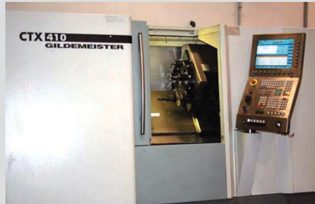
Siemens SINUMERIK 840D CNCs control the operation of the DMG machines at Smith's Machine.
