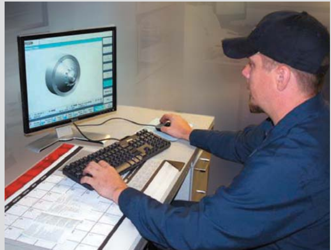
Utilizing Siemens ShopMill and ShopTurn software suites, the Smith's engineers can create programs and run actual 3D part machining simulations offline on a PC.
